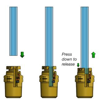
Once the tubing is connected to the fitting, make sure that the tubing is not pulled or stretched and that the minimum bend radius stated in the tubing section of this catalog is not exceeded.
