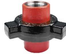
Figure 400 Threaded 4000 PSI CWP Medium Pressure Union
