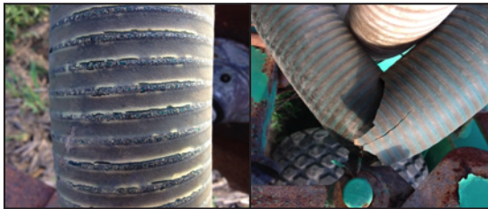
PVC Hose cracking due to UV exposure
