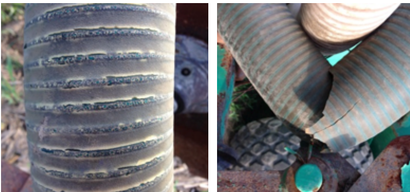
PVC Hose cracking due to UV exposure
