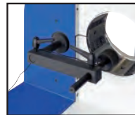
Back Limit Switch
